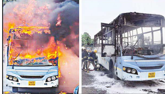
A government bus suddenly caught fire due to an electrical short circuit while traveling along a temporary service road near the Nallur railway crossing, close to Kurumbur in Thoothukudi district. More than 40 passengers escaped unharmed.
